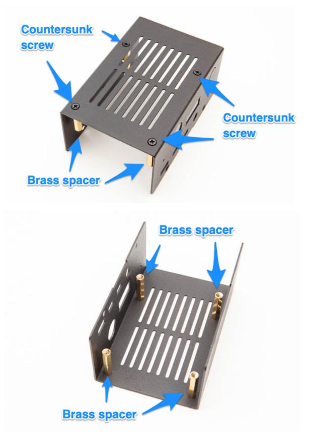
Turn the PiCAN-M board upside down and place on top of the brass spacers. You may need to push the side wall out slight in order to lower the board in place.
