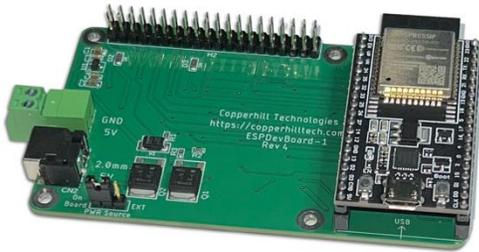
The *espBerry* DevBoard combines the [ESP32-DevKitC development board](#) with any Raspberry Pi HAT by connecting to the onboard RPi-compatible 40-pin GPIO header.
