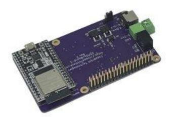
The *espBerry* DevBoard combines the <u>ESP32-DevKitC development</u> <u>board</u> with any Raspberry Pi HAT by connecting to the onboard RPicompatible 40-pin GPIO header.
