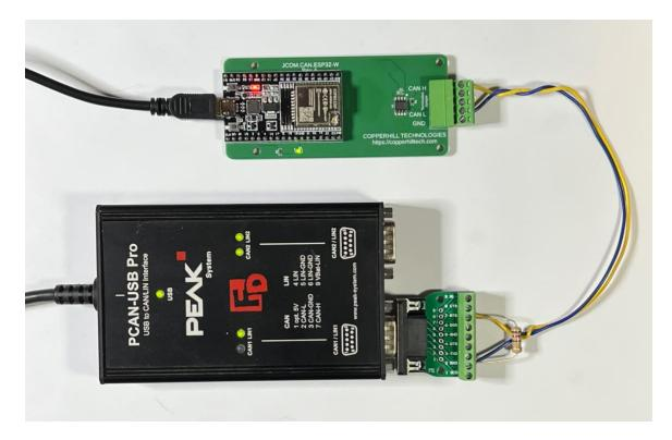
Both devices are terminated with a 120 Ohm termination resistor.  $CAN_H = Yellow - Pin 2$  on the DB9 connector  $CAN_L = Blue - Pin 6$  on the DB9 connector
