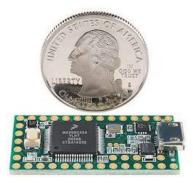
Teensy is a line of hardware boards designed to offer maximum I/O capabilities, backed up by a slew of fully featured software libraries designed to run on Arduino. The Teensy is a complete USB-based microcontroller development system, in a very small footprint, capable of implementing many types of projects. All programming is done via the USB port. The Teensy boards are fully compatible with Arduino Software & Libraries.
