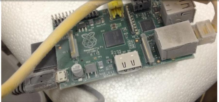
Once the tub was submerged, the temperature of the board initially dropped down to  $-78^{\circ}\text{C}$  before it stopped responding. However, removing the board and replacing it after 30 seconds saw the temperature drop to  $-82^{\circ}\text{C}$  and then  $-87^{\circ}\text{C}$  before the Pi stopped working again. At its limit the Raspberry Pi continued to function right up to  $-110^{\circ}\text{C}$ , and then started working again once it had warmed back up.
