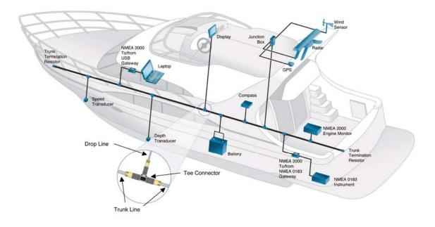
The goal of the standard is to facilitate interconnection and interchangeability between equipment from different manufacturers. NMEA 2000 is a CAN (Controller Area Network) standard which is similar to network standards that have been in use in the automobile industry for some years, and the hardware has been proven in the automobile environment.
