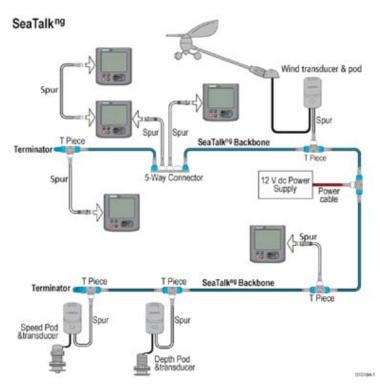
Transducer pods are offered that connect to conventional depth, speed or wind transducers on one side, and a SeaTalk NG network on the other side. These allow boat owners to convert to NG without needing to replace the transducers.
