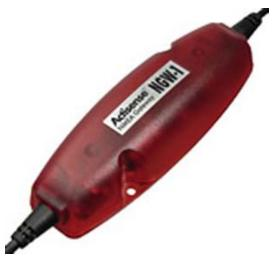
Another type of gateway will be one that connects an NMEA 2000 network to a PC using an input such as the USB connector, to feed network data to applications running on the PC.
