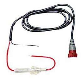
Some Lowrance displays have an NMEA 2000 power output cable. This can be connected to the network using one of the two methods above. Using this power source, which is fed by the same breaker as the display, eliminates the need to run a separate power cable to a breaker for the network. The network will always power up when the display's breaker is turned on.
