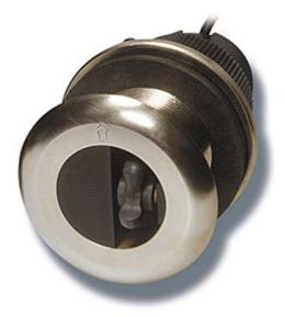
Depth and speed thru-hull or transom-mount transducers will no longer have cables that need to be run through the boat up to a dedicated display head, as is the case with most instruments today. An NMEA 2000 transducer will have a short length of drop cable attached and this will plug into the backbone as it passes by. The circuitry needed to convert the transducer data into numerical values that can be displayed will no longer be in the instrument display head, but in the transducer casing.
