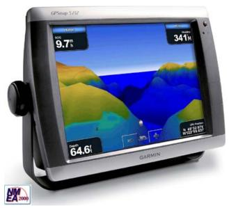
As the network can carry commands as well as sensor data, multi-function displays will evolve into boat-wide command centers which allow any device connected to the network to be turned on or off, or to be controlled. For example, an inverter could be turned on, or a VHF radio could be switched to another channel, or the audio system
