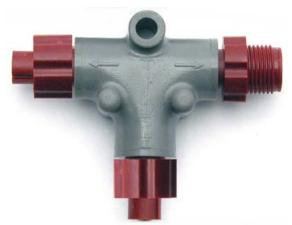
The side of the T to which the drop cable will attach is always female i.e. drop cables should have male sockets on the end that attaches to the T on the backbone. Devices that do not have drop cables permanently attached should have a male port on the back of the device. The female end of a cordset plugs into the back of the device, and the male end of the cordset plugs into the T on the backbone.
