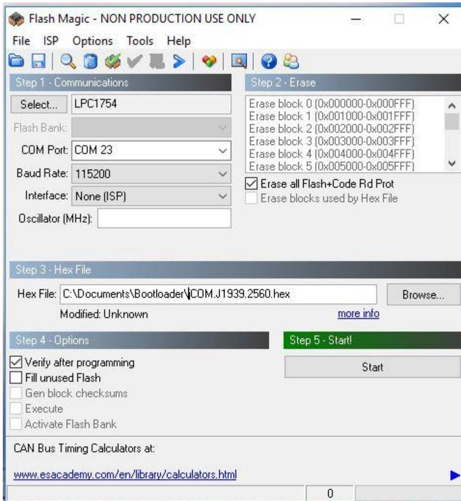
The above image shows the settings you need to apply. The only difference in your setup would be the choice of COM Port and the location and name of the .hex file.
