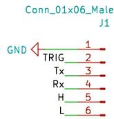
The TRIG pin is controlled from GPIO2 on the Pico. This can be driven by software to trigger a test instrument when certain conditions are observed. It can also be used as a general-purpose debugging pin (e.g. for measuring the execution time of sections code code).
