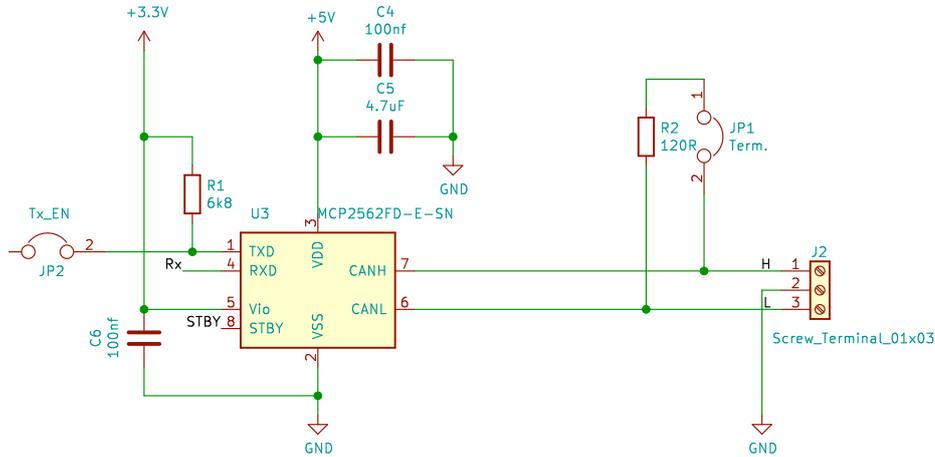
The TXD input to the transceiver comes from either the CAN controller or a GPIO pin from the Pico (the latter is to allow software to emulate aspects of the CAN protocol). The signal goes through jumper JP2 (“Tx\_EN”): if this is not closed then a pull-up resistor holds TXD high and no software can send signals on the CAN bus (this is useful if software on the Pico is to monitor a CAN bus without the possibility of disturbing it).
