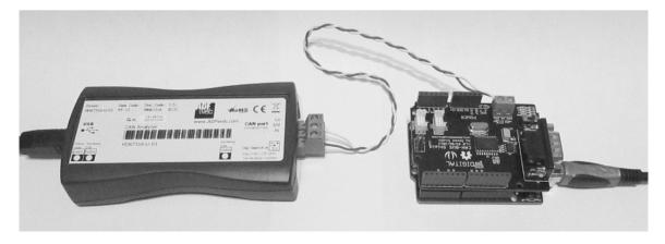
In order to test and verify the proper transmission and reception of CAN messages, I used the ADFweb CAN-to-USB gateway with its Windows interface.
