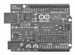
In order to develop and test the sample programs (sketches) as shown in this book, I used the Arduino Uno. The hardware consists of an open-source hardware board, usually designed around an 8-bit Atmel AVR microcontroller with 2 KB RAM (working memory), 32 KB Flash Memory (sketches) and 1 KB EEPROM (non-volatile).
