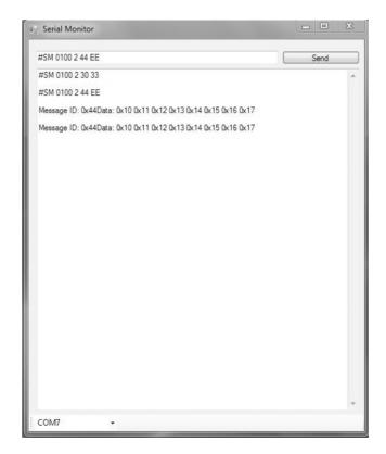
In this case, we sent two CAN Messages with the same ID (0100) but different data. Next, we received to messages through my standard test configuration (i.e. USB-to-CAN gateway with Windows monitoring tool as the second CAN node).
