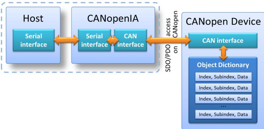
Read or write request to a remote Object Dictionary of a node on the network
